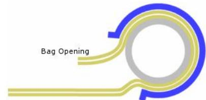
For additional clamping strength, you can attach spring clamps over the C-channel. This is not necessary under normal conditions but it will provide a better seal if the bag is heavily worn. For the ultimate gripping strength, the bag may be rolled over the tube twice before the C-channel is attached. We do not recommend more than a double roll over the tube due to the difficulty of removing the closure under such clamping pressure.
