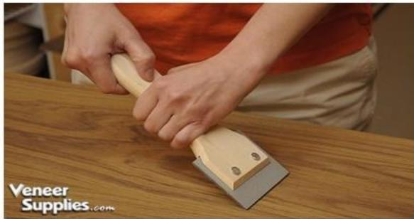
Figure 1: Scraping the veneer is critical to success.
