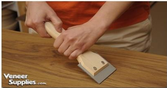
Figure 1: Scraping the veneer is critical to success. Always scrape along the grain. Scraping across the grain will cause the veneer develop bubbles.
