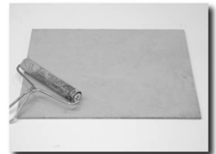
Glue applied to substrate
