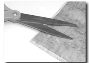
Cut off the veneer edges
