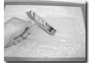
Application of glue to veneer
