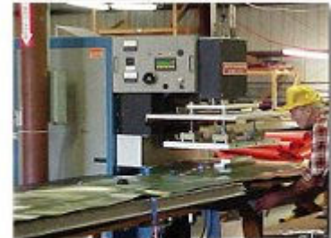
Dura-Max Vacuum Bags: Welded with 7,000 Watts of Radio Frequency
